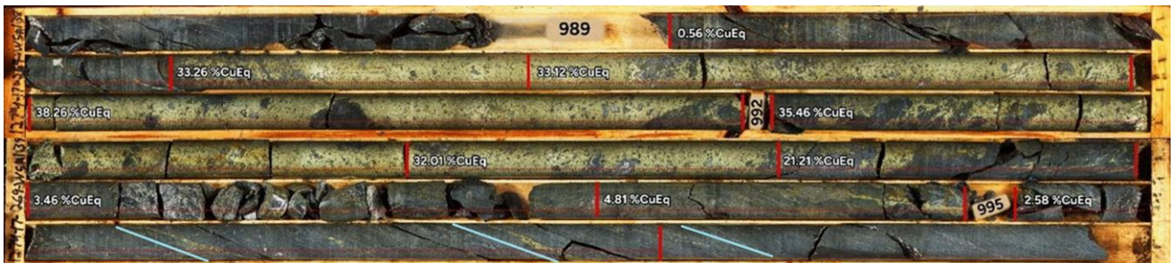
Core picture 17.91% CuEq (13.48% Cu, 5.15g/t Au) over 6.3 metres in hole 1274-17-269W5.
