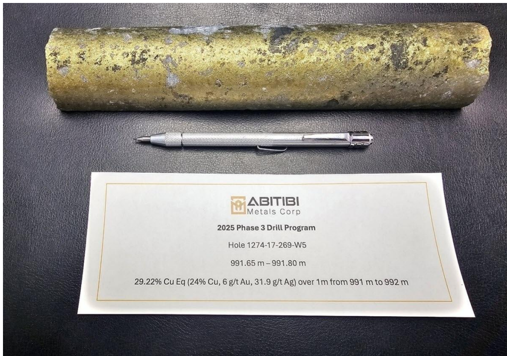
Massive Cu-Au-rich mineralization from Hole 1274-17-269W5, highlighted by 29.22% CuEq over 1m (991–992 m depth)
