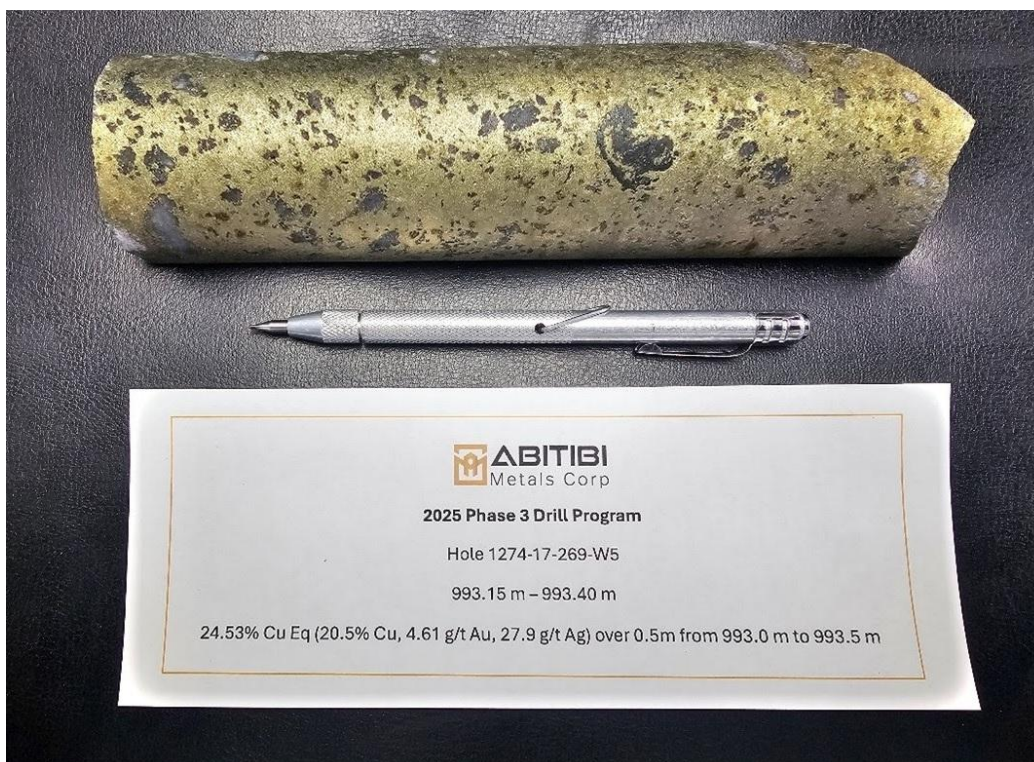
Massive Cu-Au-rich mineralization from Hole 1274-17-269W5, highlighted by 24.53% CuEq over 0.5m (993.0–993.5 m depth)
