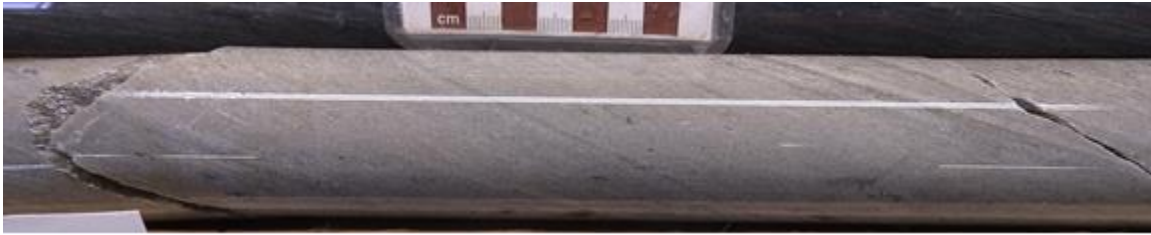
Figure 7-22 Felsic Intrusion with Quartz and Feldspar Phenocrysts, Moderate Alteration to Sericite and Weak Alteration to Chlorite, Drill Hole 1274-16-230 at 336 m
