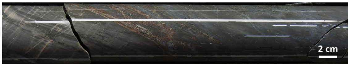
Figure 7-37 Veinlets of Sphalerite-Pyrite in the Aphyric Rhyolite, Drill Hole 1274-17-259 at 490 m
