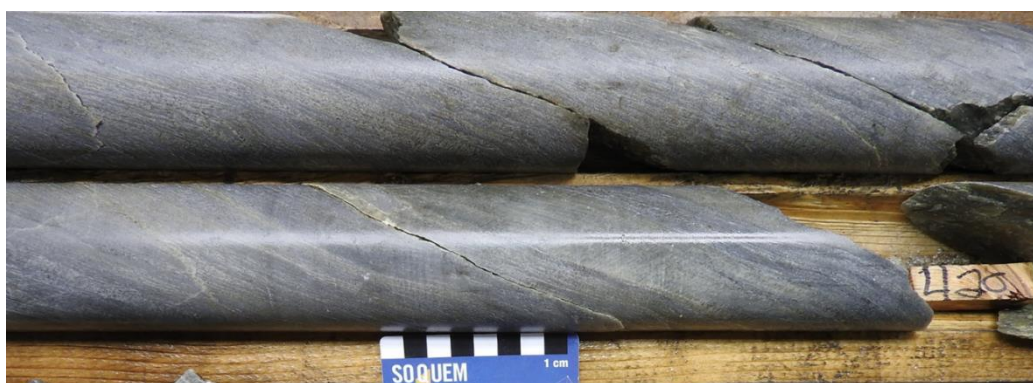
Figure 7-33 Intense Sericite Alteration Overlying the Brecciated Aphyric Rhyolite, Drill Hole 1274-17-259 at 420 m
