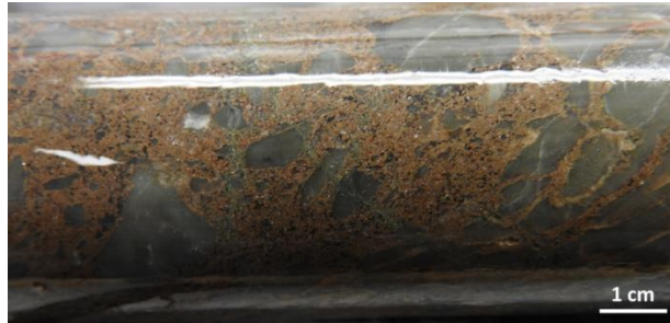
Figure 7-38 Sphalerite-Pyrite-Galena-Ag Breccia in the Aphyric Rhyolite, Drill Hole 1274-17-249 at 500 m
