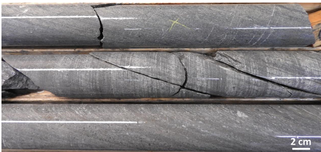
Figure 7-14 Felsic Tuff with Quartz Crystals and Lapilli, With Beds and Laminations of Massive to Disseminated Pyrite, Drill Hole 1274-16-235 at 646 m
