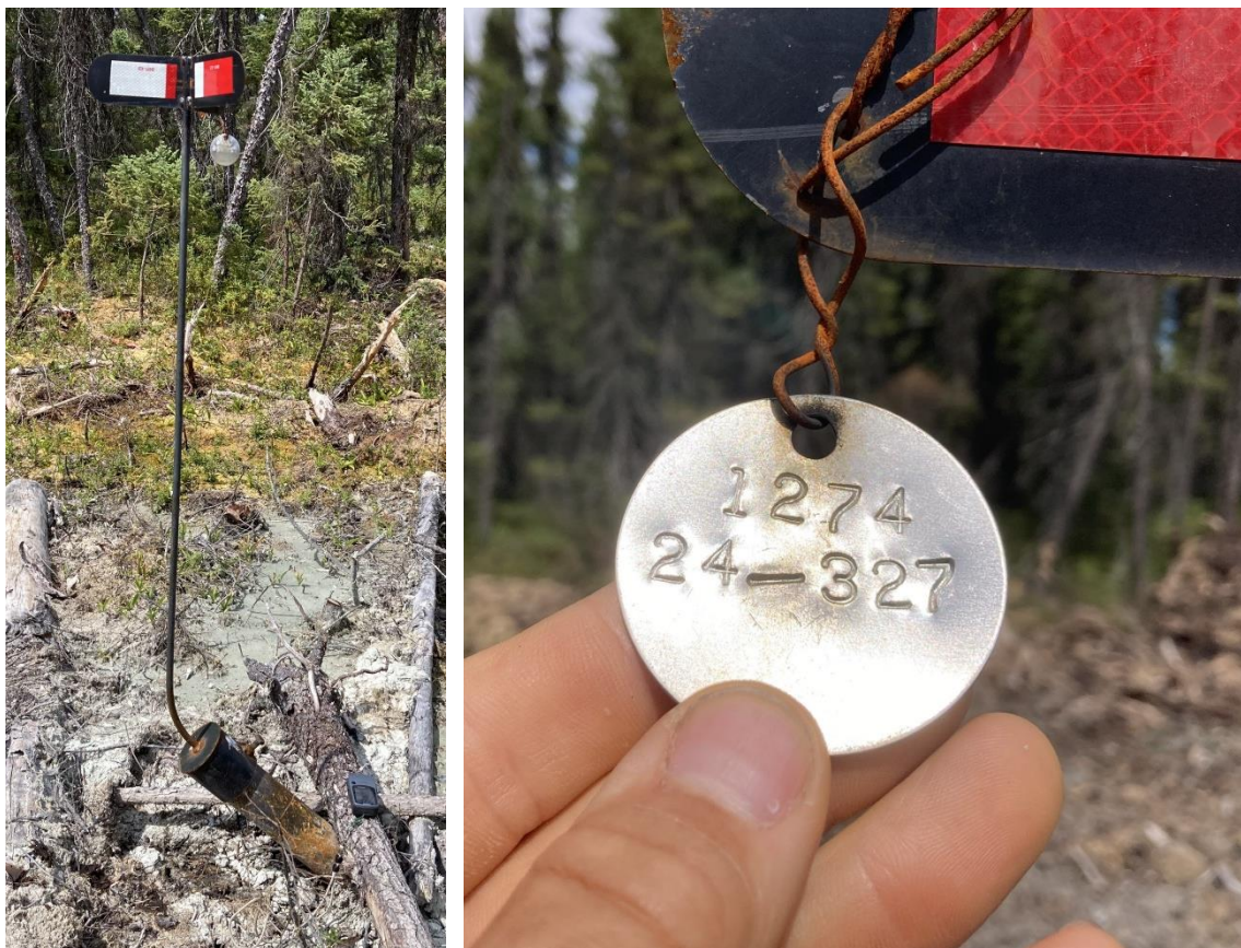
Figure 10-1 Example of Drill Casing, Marker and Identification Tag with Drilling by Abitibi Metals
