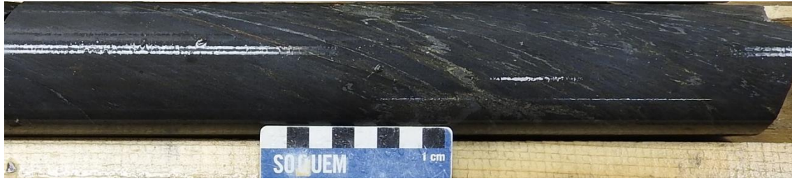
Figure 7-29 Folded Veinlet of Ankerite-Magnetite-Pyrite in the Aphyric Rhyolite, Drill Hole 1274-17-252 at 436 m
