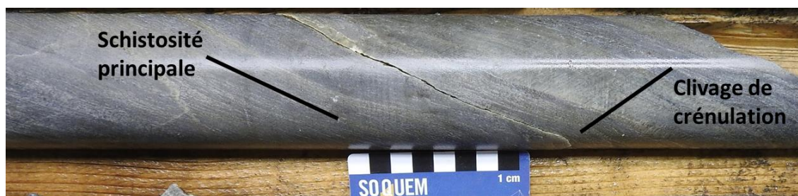
Figure 7-27 Main Schistosity Plane and Crenulation Cleavage in Altered Aphyric Rhyolite, Drill Hole 1274-17-259 at 420 m
