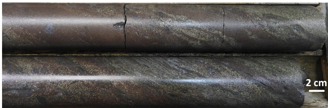
Figure 7-36 Lenses of Massive Sulfides (Top) to Semi-Massive (Bottom), Drill Hole 1274-17-259 at 453 m
