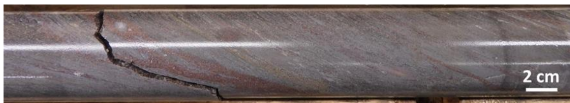
Figure 7-11 Massive Sulfide Replacement Containing Fragments (Center) with Sub-Concordant Laminations of Semi-Massive Sulfides (Bottom), Drill Hole 1274-16-224 at 403 m
