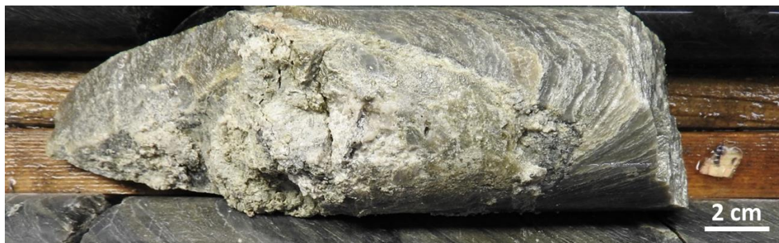
Figure 7-28 Decimetric-Thick Fault Cutting through Altered Aphyric Rhyolite. The Fault Plane Has Rotated 45° Clockwise Relative to the Main Schistosity Plane when Looking towards the End of the Hole, Drill Hole 1274-17-252 at 337 m
